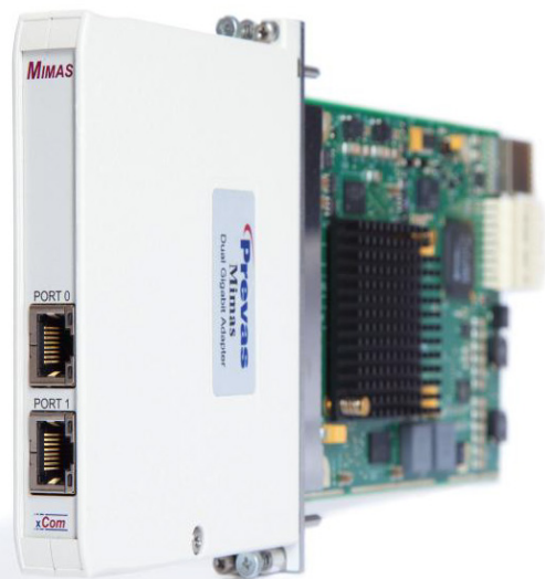
Prevas' Mimas connected to NI's FlexRIO module
