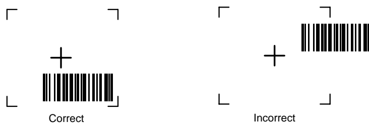
Figure 2-20 Imager Aiming Pattern: Bar Code Not Centered
